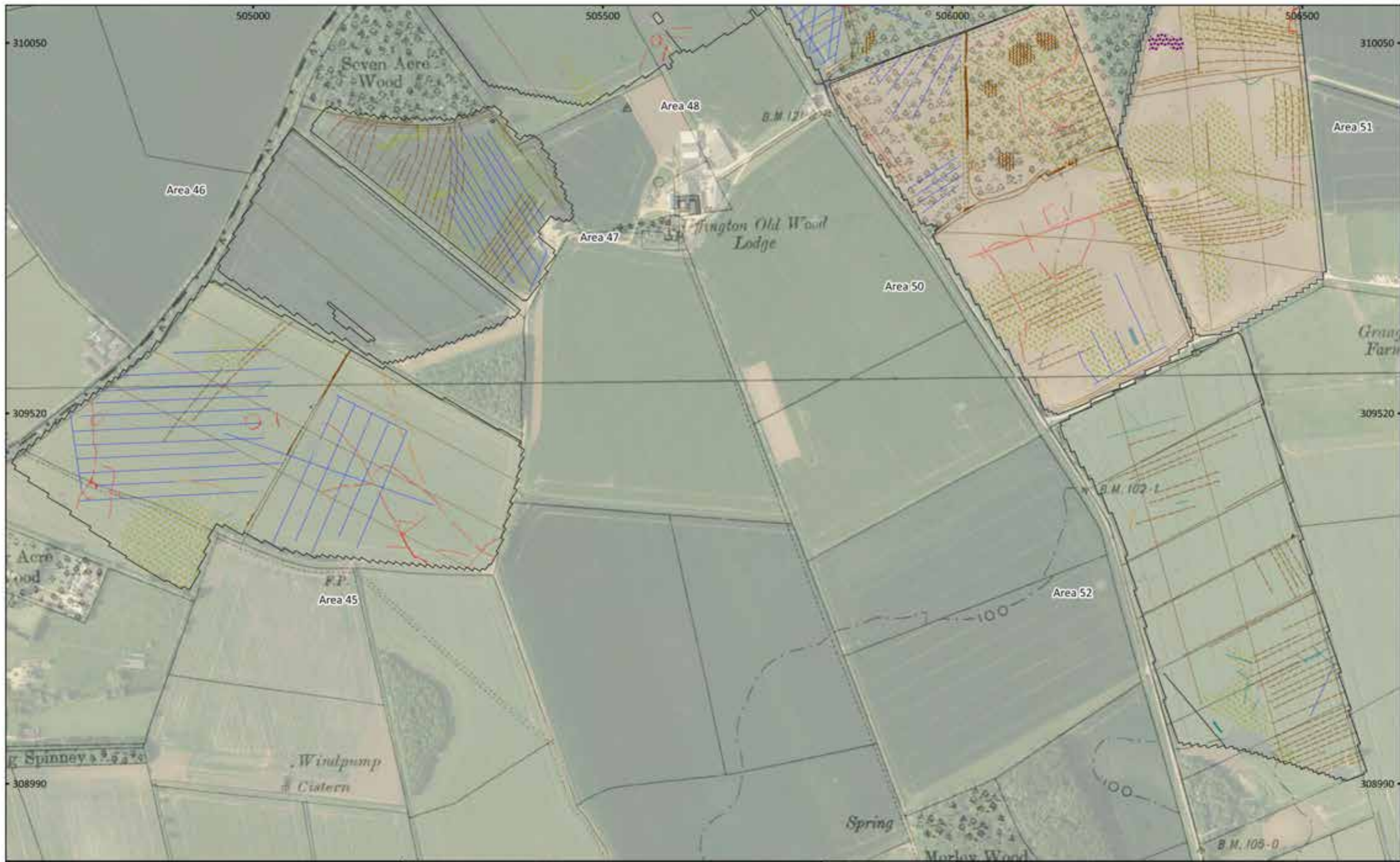
MSTF1136: Mallard Pass, DCO, Essendine, Rutland Figure 22 - Magnetic Interpretation Over Historical Maps and Satellite Imagery 1:5,000 @ A3 Copyright Magnitude Surveys Ltd 2022 Contains historical mapping © CLS Data 2022: Ordnance Survey, 6" 2nd edition c. 1882-1913 Contains satellite imagery © Bing Satellite 2022
